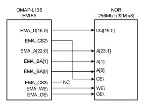
Figure 5. Hardware Connection for 16 M x 16 Device
