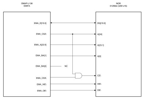
Figure 6. Hardware Connection for 32 M x 16 Device
