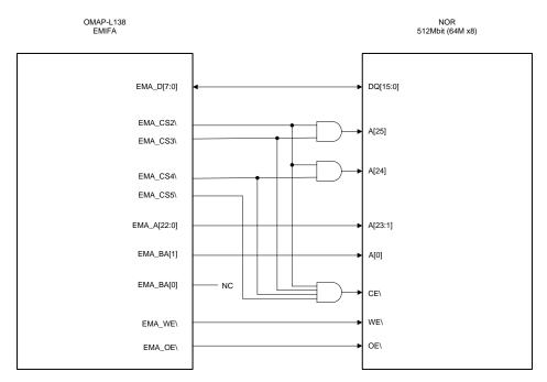
Figure 8. Hardware Connection for 64 M x 16 Device
