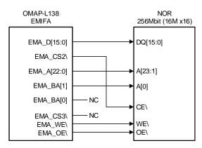
Figure 4. Hardware Connection for 16 M x 16 Device
