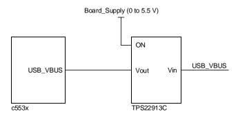
Figure 3. Isolation Circuit for Device-Only Mode
