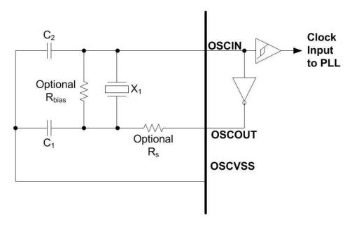
Figure 1. Crystal Circuit
