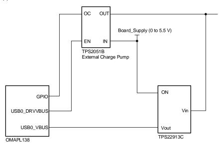
Figure 2. Isolation Circuit for OTG Host/Device Mode
