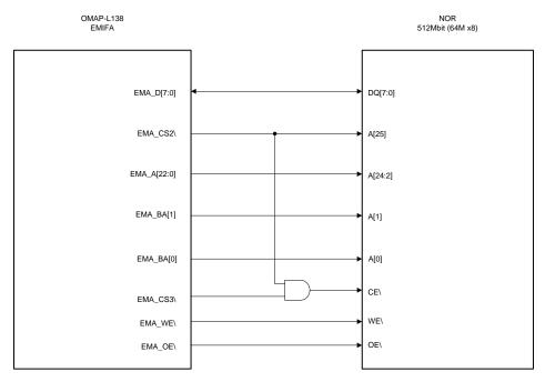
Figure 7. Hardware Connection for 64 M x 8 Device
