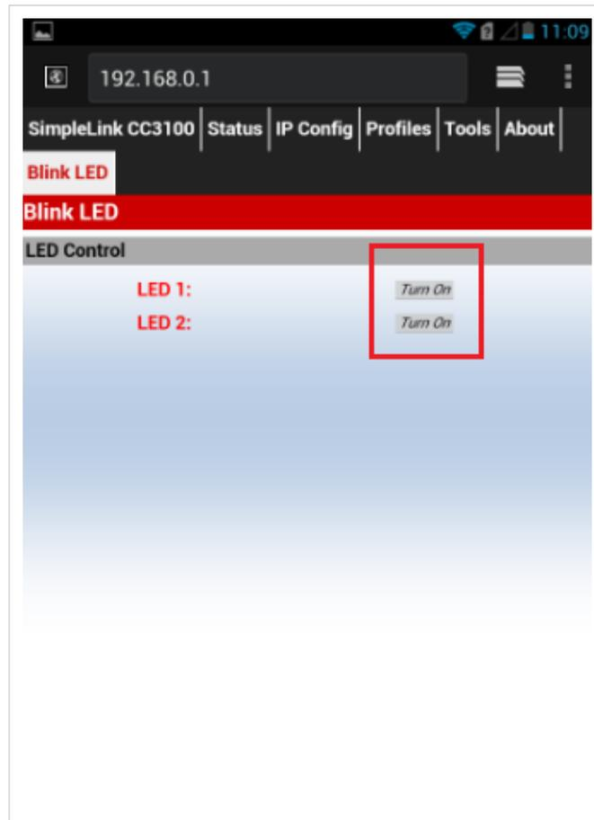
**Note:** : User needs to reconfigure the device in 'Station-Mode' for executing other sample applications. Refer function `configureSimpleLinkToDefaultState` in this example's `main.c` for configuring the device in 'Station-Mode'.
