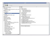
While still in xconfig you can change the SDRAM, ZRELADDR, PARAMS\_PHYS, and INITRD\_PHYS locations for you memory map. For example to allocate 16MB of memory at the beginning of DDR for the DSP image you can double click on each item and change the value. Press ENTER to save each value. i.e.
